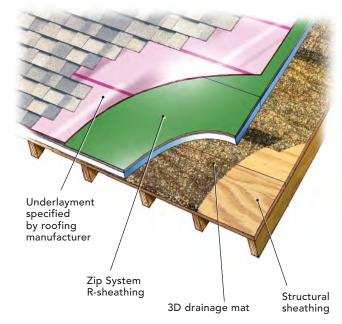
between the structural roof sheathing and the R-sheathing and an additional roofing underlayment, as specified by the roofing manufacturer, on top of the R-sheathing. In this application, R-sheathing is to be screwed to the roof deck and to the framing with "code recognized nail base fasteners," including FastenMaster HeadLok, Simpson Strong-Tie SDWS, and similar structural fasteners.
