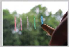
The best by far for glass. Wax pencils make clear marks on glass that are durable but also easily removed with solvent.
