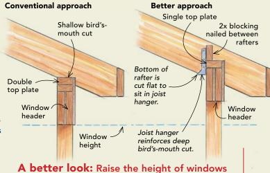
This often-seen and, in my opinion, always ugly detail (above, left) has become the conventional approach to building the front edge of the dormer roof. It's easy to frame, but it forces you to lower the windows to accommodate the header. But by cutting a deep bird's mouth in the shed rafter and capping the wall with a single top plate, I can move up the header and raise the window height.
