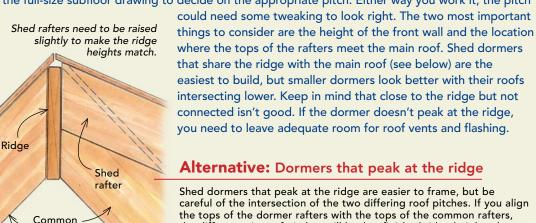
the tops of the dormer rafters with the tops of the common rafters, the difference in roof pitches will lead to finished ridge heights that don't match. Raising the shed rafter slightly solves the problem.
