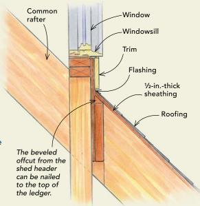
Stop the sheathing at the roof ledger; otherwise the space under the short front roof is impossible to insulate properly.
