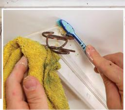
**Wet cleanup.** Use a damp rag and toothbrush to clean wood glue squeeze-out from joints while it's still wet.
