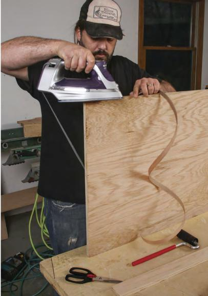
Band the edges. You can conceal plywood edges with solid stock, or you can use edgebanding tape with hot-melt glue on the back. The glue is heated with a clothes iron, and then the edgeband is rolled with a laminate roller.
