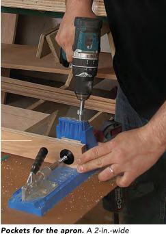
Pockets for the apron. A 2-in.-wide plywood apron hides the desk's steel reinforcement. It's fastened to the bottom of the desktop with screws in closely spaced pocket holes drilled using a pocket-hole jig.
