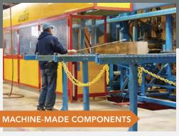
Most frame parts are cut to length and the joinery is made with a German-made Hundegger K2i CNC joinery machine, but the machine-cut joints often need corners squared and stray wood fibers trimmed.
