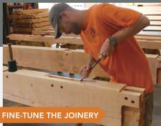
Joinery and cuts are fine-tuned and chamfered with traditional timber-framing tools, including block planes, chisels, and mallets. The heavy timbers are handled with forklifts to boost efficiency and prevent injury.
