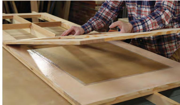
Roll on the glue. I recommend using Titebond III glue, which is waterproof and has a long open time ideal for a complicated glue up. Use a mini paint roller to apply a thin coat onto both mating surfaces, overlapping the edges of the MDO panel.
