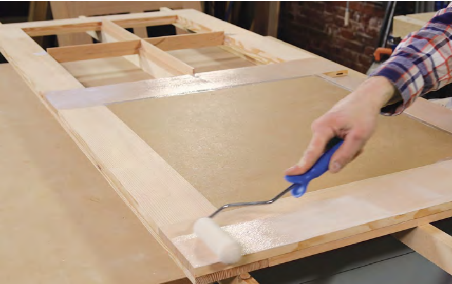
Roll on the glue. I recommend using Titebond III glue, which is waterproof and has a long open time ideal for a complicated glue up. Use a mini paint roller to apply a thin coat onto both mating surfaces, overlapping the edges of the MDO panel.
