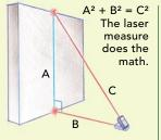
store measurements, add and subtract consecutive measurements, and add and subtract against a constant measurement. Most models also perform continuous measurements, which allows you to move the tool toward or away from a target while the changing distance is shown on the screen.
