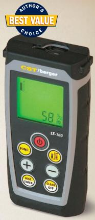
Accuracy. The first thing I would look for is the highest stated accuracy I could afford. All the tools here other than the Craftsman are accurate to within 1/16 in. over their maximum distance, more than adequate for any carpentry task. There are less accurate (and less expensive) models; they would be fine if you are just estimating.
