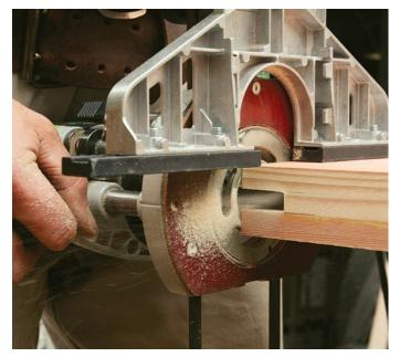
**2** Cut the groove with multiple router passes. The Pemko mechanism requires a groove %6 in. wide and 1%6 in. deep. After fitting a ½-in.-dia. bit (www.freud.com) in my router, I attach and adjust a fence to center the groove in the door's bottom edge. Then I rout the groove in multiple passes, increasing the cutting depth ¼ in. to ¾6 in. each time. I widen the groove to ¾6 in. by adjusting the router fence on the final pass.
