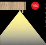
A well-placed shallow recess allows light to spread out across the counter and puts the bright spot right where it's needed.
