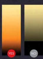
MLV) dimmers work for most controls; 010v and DMX, a digital language, are for very precise dimming control. Warm-dim tape is ideal for shifting warm white (2700K) to very warm (1800K) as it dims.
