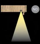
Deep recesses or frames shield fixtures but leave deep shadowlines on the counters.
