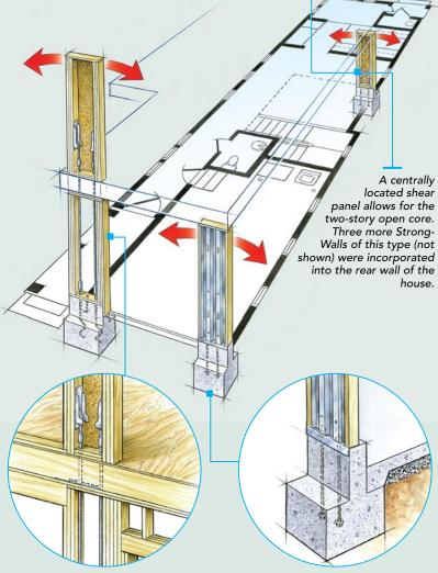
Connected to the foundation with 1-in.-dia. steel rods, a second-floor Strong-Wall secures the structure against the seismic and wind-shear loads that a tall, skinny building might encounter.
