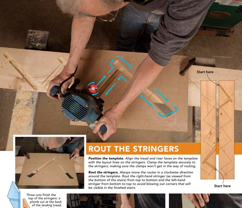
Three cuts finish the top of the stringers: a plumb cut at the back of the landing tread, another plumb cut at the back of the riser, and a level cut at the bottom of the landing tread.
