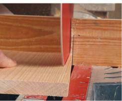
**Cut the wedges.** Set the miter saw's table to 2° and cut with the grain. Flip the board end for end, cut again, and the resulting wedge will have a 4° slope. Use a zero-clearance fence, and mark the width of the wedge's skinny end on the fence for consistency.
