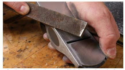
**Soften the edges.** Unlike a larger plane, a block plane is small enough to fit in one hand. Make the planing experience more comfortable by easing the edges with a file. Doing this file work on the bottom edges will also help the plane glide more smoothly on the wood.
