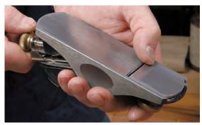
**Straighten the blade.** After sharpening, install the iron and either sight down the sole or feel with your fingers to be sure the cutting edge is parallel to the mouth. Some planes have an adjustment lever for this and others require tapping the blade to and fro until you get it parallel.
