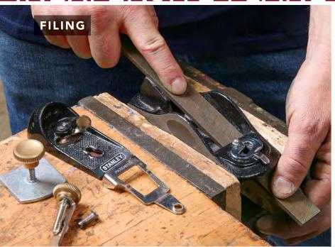
**Smooth the bed.** Burrs from the machining process and paint overspray will prevent the blade from sitting flat on the bed. Smooth these inconsistencies with a fine file. Also look at the bottom of the lever cap and file it flat where it contacts the blade. Finish by cleaning and oiling the adjustment screws.
