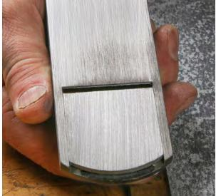
Focus on the mouth. Ideally, the entire surface of the sole is evenly abraded. But at a minimum, you want the area directly in front of the cutting edge to be flat and a good percentage of the rest of the sole flat as well. When the bottom shows nearly uniform scratch marks, switch to 220-grit paper and sand again until the sole shows a uniform polish.
