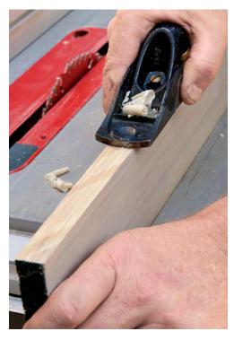
Your block plane offers a fast and quiet way to remove saw marks
