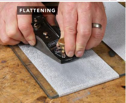
**Flatten the sole.** Retract the blade and lock it in place. Then, with even pressure, swipe the sole back and forth over 120-grit or 150-grit sandpaper adhered to a piece of glass or granite, or a cast-iron machine surface.
