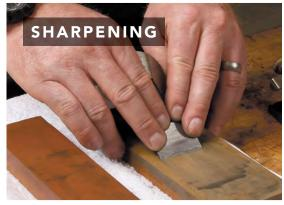
Hone the blade. Once the plane body is tuned, hone the blade with diamond stones or water stones. If you want to soup up your old or less expensive plane, buy a replacement blade from Hock Tools (hocktools.com). These high-carbon-steel replacement blades get sharper and hold an edge longer than most stock irons.
