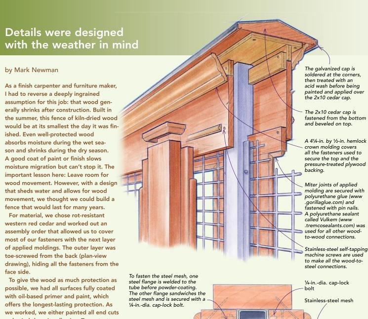
or buried them in adhesive. To protect the top, we sloped the cap with a 5° bevel to shed water and added a galvanized sheet-metal cap.
