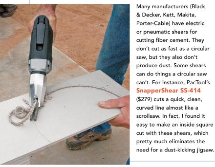
Many manufacturers (Black & Decker, Kett, Makita, Porter-Cable) have electric or pneumatic shears for cutting fiber cement. They don't cut as fast as a circular saw, but they also don't produce dust. Some shears can do things a circular saw can't. For instance, PacTool's **SnapperShear SS-414** (\$279) cuts a quick, clean, curved line almost like a scrollsaw. In fact, I found it
