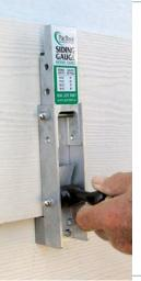
PacTool has both metal and plastic siding gauges (metal, \$79; plastic, \$59) that slip under the bottom edge
