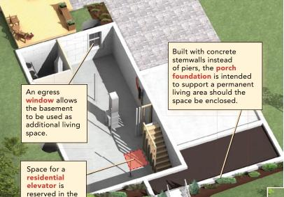
Construction detail: The foundation was built using American PolySteel insulating concrete form (ICF) panels. These large ICFs were preassembled off site under tight quality-control measures. The ease and speed with which they can be assembled allowed the construction crew to build and pour the foundation in only one day. www.polysteel.com
