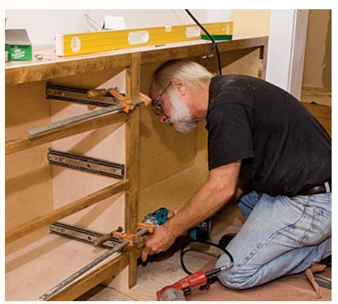
First assembly is done in the shop for a better final fit. After Jerry Nees glued the center face frame to the center cabinet, he clamped the base cabinets together in the shop. The left and right portions of the face frame then can be scribed to fit and glued to their respective cabinets. The process is repeated for the upper cabinets.
