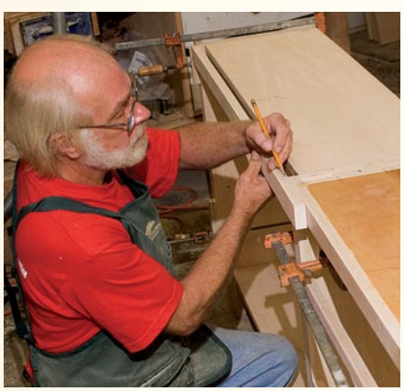
First assembly is done in the shop for a better final fit. After Jerry Nees glued the center face frame to the center cabinet, he clamped the base cabinets together in the shop. The left and right portions of the face frame then can be scribed to fit and glued to their respective cabinets. The process is repeated for the upper cabinets.
