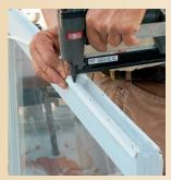
here, is designed to sit in a groove. While this is usually a good approach, it did not work for this application. The wide rope channel left little "meat" along the stiles to run the groove, and the seal would have stood proud of the interior stop, which my client did not want.
