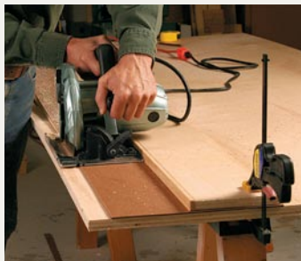
Cutting plywood can be unwieldy. Sometimes the best solution is to cut it with a circular saw guided by a fence.
