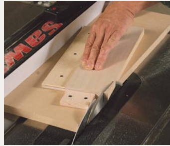
Cutting tapers. A pair of stop blocks screwed to a wooden sled position the tapered leg as it passes over a tablesaw blade.
