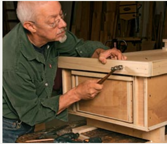
Trim the top first. The 1½-in.-thick rim pieces at the top of the base box rise ¾ in. above the plywood to retain the cushion.
