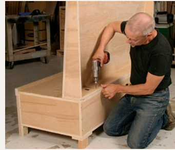
Attach the backrest. Screw the tapered box to the base box. Avoid screw points extending into the drawer section.
