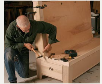
Clamps help. Test-fit the top and side trim pieces, and clamp them together to ensure a tight fit as the nails are driven home.
