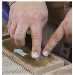
Polish the microbevel. Repeat the sharpening process on each of the polishing blocks. Remember to wipe off the chisel between each one.
