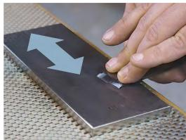
5 Side to side. Flatten the back of the chisel by stroking it side to side on the 300-grit side of the plate until the back of the tool is perfectly flat at the leading edge. Then use the 1000-grit side of the plate to remove scratches left by the coarser side of the plate. You shouldn't have to flatten the back of the chisel again unless it gets damaged from use.
