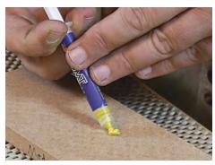
A little bead is all you need. Press a pea-sized amount of diamond paste into the center of the block. If your blocks stay clean and free of debris, you won't have to add more paste for a while. When it begins to take a long time to polish your tool, recharge the blocks with more paste.
