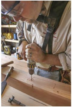
**Start small.** After scoring the perimeter of the mortise, use a small-diameter drill bit to remove material from each of the four corners, which will be out of reach of the larger bit that comes next.
