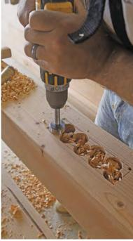
**Clear the waste.** Use a Forstner bit to hog out the mortise and leave a flat bottom. For consistent depth, chuck the bit so that it sticks out only as far as the mortise is deep.
