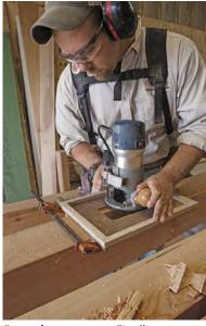
**Rout the recesses.** Finally, use a template and pattern bit to rout a shallow recess, sized to match the adjoining timber, around the perimeter of the mortise.
