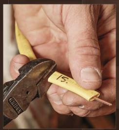
Save the label. Clip off the label and set it aside, then peel the sheathing and paper off the wires, and use diagonal cutters to cleanly cut them from the wires.
