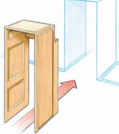
**Tilt and slide.** After the original head jamb and top panel are attached to the side jambs, I tip up the unit, center it in the rough opening, and slide it in place. An extra set of hands ensures that the unit won't rack as it's positioned.
