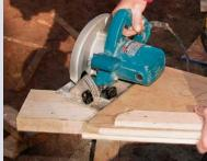
**Tip:** Stop the fence short of the jig's plywood edge. This way, the saw can clear when you use the jig as a saw guide for plumb cuts.
