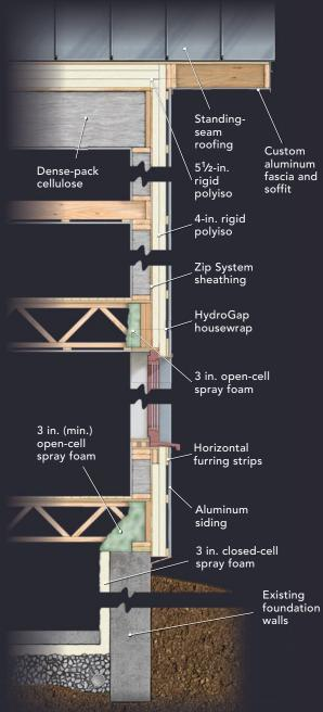
dense-pack cellulose inside the stud cavities and two layers of 2-in. fiberglass-mat-faced polyisocyanurate rigid insulation outside. The R-70 roof assembly has 12 in. of dense-pack cellulose in the rafter cavities, and two layers of 2-in. and one layer of 1½-in. mat-faced polyisocyanurate rigid insulation above the roof deck.
