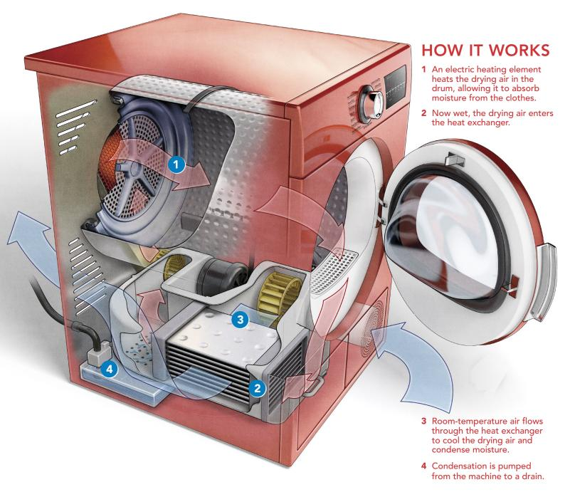
ost dryers sold and installed in the United States continuously draw fresh air from the laundry room, heat it before it picks up moisture from the wet clothes, and then vent the hot, moist air out of the house. Not only is this a literal energy suck, but if you don't have the space for lengthy ductwork or want to locate your laundry room against an interior wall, you'll have to make a choice: hang a clothesline, or go with an unvented dryer.
