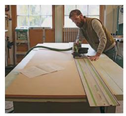
All from a single sheet. All of the MDF parts for this project come from a single 4x8 sheet. They are first broken down by width using a tracksaw, then taken to the miter saw to be cut to length.
