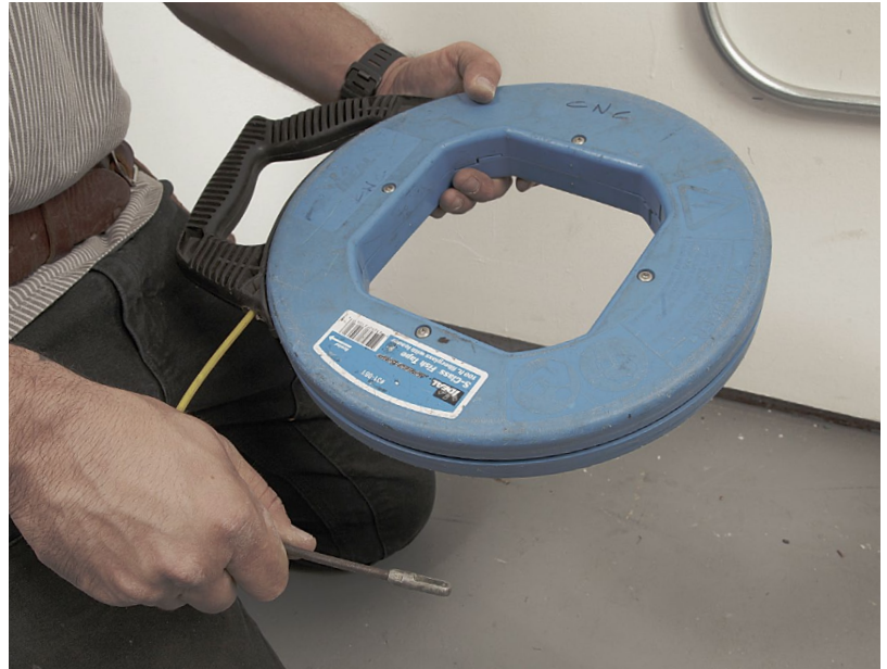
Fish-tape anatomy. My fish tape has an eyelet end, rather than a leader, as some tapes have. I prefer this because it's a solid piece that can't spring apart. My Ideal S-Class fish tap costs about $175.
