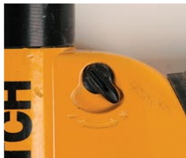
The adjustable power level (depth of drive) was largely unnecessary.
