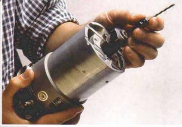
Converting a standard router for drywall use. A '/a-in. adapter chuck and a drywall bit are all it takes to set up a standard router for drywall (photo above). To cut out for doorways (photo left) and electrical boxes (photo below), the author uses a piloted bit, which spins alongside the underlying surface without damage or binding.
