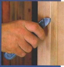
Renewing a tired blade. Cutting drywall wears out knife blades quickly. The standard alternative to replacing a dull blade is to resharpen it on a pocket stone (top photo). A more radical, faster approach is to snap off the worn end to access the unused inner part of the blade.
