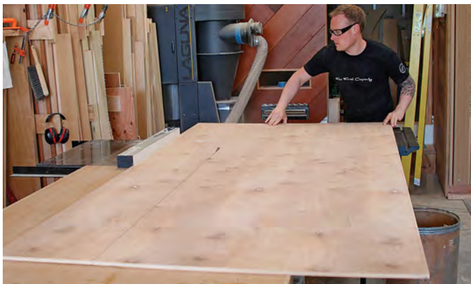
Start ripping. Rip panel stock to width on a tablesaw before cutting it to length. Plan your cuts to use the stock efficiently, and rip like-size panels all at once to save setup time.
