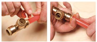
To remove the fitting, place the removal tool over the tubing, and press it against the fitting's plastic collar until the fitting releases.
