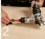
Insert the expansion-tool head into the tubing, pull the trigger to expand once; then rotate the tool slightly and expand again.
