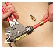
Insert the expansion-tool head into the tubing, and expand it. Release the tool, rotate it 45°, expand the tubing again, and hold it for five seconds.
