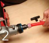
Repeat the expansion process until the tubing and ring butt up to the shoulder of the expansion head.
