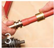
Release and remove the expansion tool, and immediately insert the fitting so that its last barb is just shy of the end of the tubing (about  $\frac{1}{16}$  in. away).
