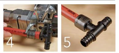
Turn the tool around and slide the compression jaws onto the fitting and tubing. Pull the trigger to pull the sleeve all the way to the fitting's collar. The tool stops and resets automatically.
