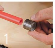
Slip a sleeve onto the tubing, sliding it back far enough that it doesn't interfere with the expansion.
