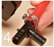
Place the tool's jaws over the clamp's tab, and squeeze until the tool releases. A mechanism prevents the tool from releasing until the connection is complete.
