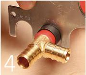
After crimping, check the result using a go/no-go gauge. If the go/no-go check fails, cut the tubing just beyond the end of the fitting, and start over.
