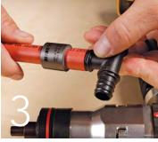
Remove the tool and immediately insert the fitting so that the tubing is snug against the fitting's stop.
