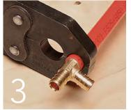
Fit the crimp tool's jaws over the ring and squeeze the handles all the way to crimp the ring into place.
