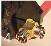
Squeeze the trigger to engage the tool and press the fitting.
