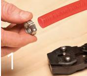
Slide a stainless-steel clamp onto the tubing.
