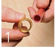
Slide a compression sleeve onto the tubing, beveled end toward the fitting, pushing it far enough so it won't interfere with the expansion process.
