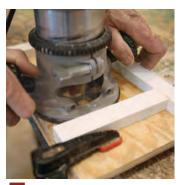
Fout the opening in the jig. After setting the bit just deeper than the plywood, clamp the jig to a scrap and rout through the jig's base, moving clockwise for a controlled cut.
