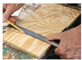
**2** Locate the side fences. Double the measurement from step 1 and add it to the hinge height to find the side-fence spacing.
