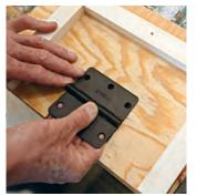
Test the fit. Right now, only the hinge height matters. To allow some vertical adjustment when hanging the door, 1/32 in. of play is perfect.
