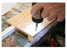
**Fasten the back fence.** To create a back fence, align a scrap of 1x to the edge of the plywood and fasten it with screws driven from the bottom of the jig.
