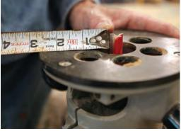
**Measure the offset.** Measure across the radius of the router base to the bit's edge. The smallest measurement is the right number.
