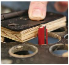
Set the cutting depth. Adjust the router's depth of cut so the bottom of the bit is flush with a hinge leaf held on a scrap from the jig base.
