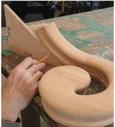
Locate the cut. Set the pitch block with the run side on a flat surface, place the fitting on the same surface, and mark the point where the two intersect. (To mark an up-easing or gooseneck, rest the pitch block on its rise side.)
