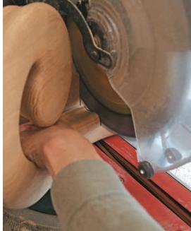
Make the cut. Make an auxiliary fence by clamping a piece of plywood or MDF to a miter saw, and make the initial cut through it. Then, hold the fitting so its bottom fully contacts the auxiliary fence, line up the mark with the kerf in the fence, and cut to the line.
