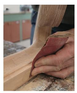
13 Fair the joint. Rails and fittings are made on separate machines and rarely match perfectly. If you're lucky, sanding will be enough to fair the joint, but most cases require a combination of chisels and files, with sanding as the final step.
