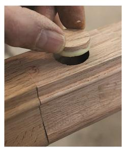
12 Plug the hole. Glue in the 1-in. plug included with the rail bolt, being sure to line up the grain direction. Leaving the plug a little proud makes it easier to flush the two up in the next step.
