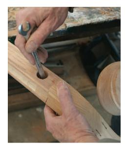
**Connect the parts.** Coat the ends of the rail and the fitting with glue, put the bolt into the rail, and place a washer and nut on the end. Keeping the beads on the rail and fitting aligned, tighten the nut with a ½-in. wrench.
