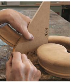
Mark the cut. Keep the fitting on the flat surface, then flip the pitch block to its rise side and use it to mark a cutline. (To mark an up-easing or gooseneck, rest the pitch block on its run side.)
