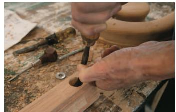
Make way for the washer and nut. Chisel a flat spot inside the access hole that's large enough to accommodate a 5/16-in. flat washer, being careful not to damage the rim of the hole. A sharp 3/8-in. chisel works well.
