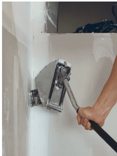
Angle box for corners. Adaptable to angle heads of various sizes, an angle box dispenses an even coat of compound to both sides of an inside corner.
