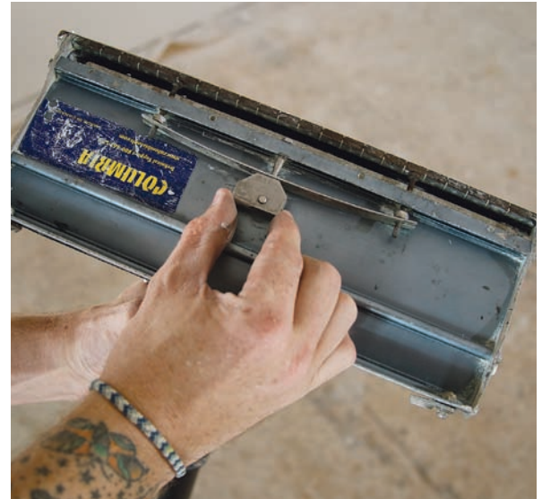
Adjust the flow. The eccentric cam adjusts the flow, so you can determine the amount of compound to dispense. The idea is to fully coat the seam without excess and leave a smooth finish free of voids as you go.
