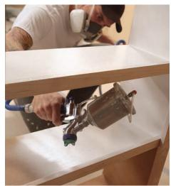
**Start upside down.** Even though all of the surfaces will be sanded, I spray cabinetry upside down so that overspray will land on what will be the underside of the shelves, where a dead-smooth surface is less crucial.
