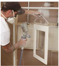
Simple spray rack. For small parts that need to be coated on both sides, I suspend the pieces from coat hangers using small hooks spun to face opposing directions, all hung from an old rolling garment rack.
