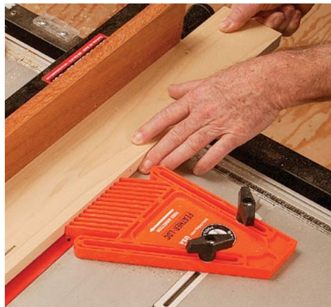
Bench Dog ( www.benchdog.com ) featherboards ride in the miter-gauge slot.
