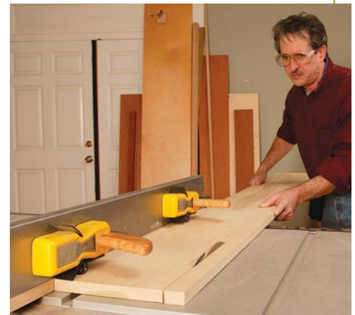
Grip-Tite ( www.grip-tite.com ) magnetic hold-downs stick to a steel auxiliary fence.
