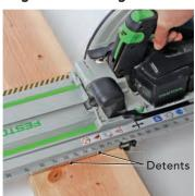
An easy-to-read scale on the left side of the track shows the angle setting for miters. The notches cut into the track are detents for common cuts.
