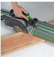
By adjusting the sliding pivot, the saw can make left and right angled cuts. The track's plastic edge lines up with the blade for accurate alignment and less splintering.
