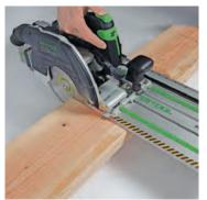
With the fixed pivot and adjustable stop tight to the stock, the aluminum track guides the saw.
