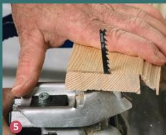
profile with the saw held at a slight angle to create a back bevel.
