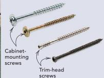
Many cabinet companies now supply mounting screws, but years ago, we were left to our own devices. Like many installers, I made the mistake of hanging cabinets with drywall screws, which simply aren't strong enough to support loaded cabinets. These days, I use only special cabinet-mounting screws, preferably those with broad washer heads for full shoulder support (www. mcfeelys.com). To join stiles, I use trim-head screws. The smaller heads can be hidden easily by hinges, plugs, or wood putty.
