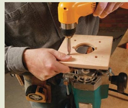
A square plywood base keeps the router parallel to the stock as it descends the ramp.
