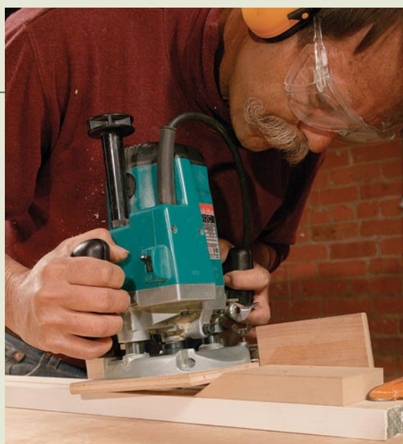
An extralarge fence keeps the router parallel to the stock.
