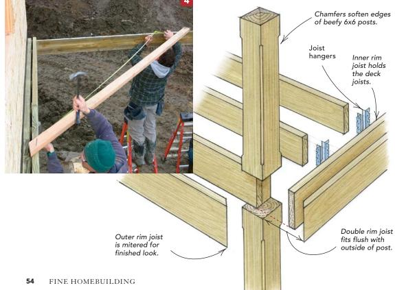
details to establish the length. Because 6x6 posts tend to look massive, I often soften the edges with routed chamfers.
