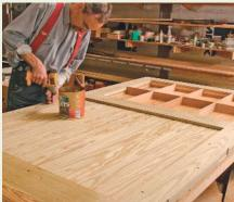
Completing the sandwich. With the exterior stile-and-rail assembly installed, the door is nearly done. The beadboard paneling and exterior frame are made from pressure-treated pine to resist mold and insect damage.
