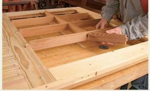
**Easy muntins.** Tenon shoulders for the muntin assembly are cut on a tablesaw; the mortises can be drilled and cleaned up with a chisel. Horizontal muntins are let into vertical muntins with mortises and stub (shortened) tenons. Added later, simple applied stop moldings will hold the glass panes in place.
