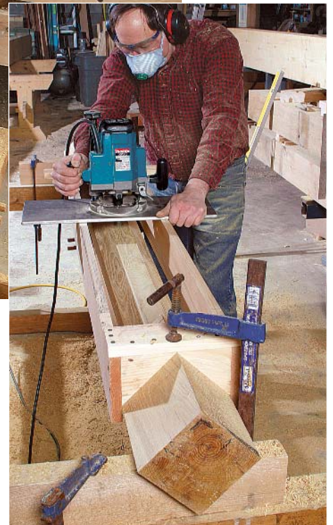
Angled sled turns four sides into eight. A sled similar to the first, except that it's equipped with 45° angle blocks, directs the router to cut the angled sides of the octagon.
