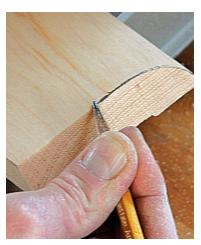
Use a pencil to highlight the cutline. To make the profile of the molding more apparent, draw the flat edge of a pencil lead across the inside edge of the miter cut.
