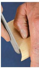
The back bevel allows minor adjustments to be accomplished using a few passes with a wood rasp rather than a belt sander.
