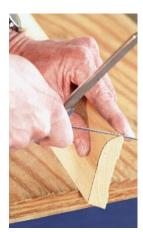
Angle the cut inward. Start the cut with a few gentle pull strokes until the coping saw finds its groove; then switch to long push strokes.
