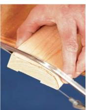
Angle the blade into the work so that the face of the cut becomes slightly proud of the back side. This slight angle is called a back bevel, or back cut.
