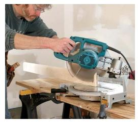
Miter cut determines the profile. Although you can trace the profile from one piece of trim to the other, a 45° inside miter cut achieves the same purpose. An efficient carpenter chops all the profiles for a particular room at the same time, then cuts each piece of trim to length later.
