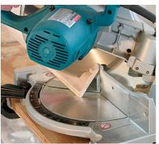
Place the crown molding upside down in the miter saw and at an angle between the fence and base. Then make a 45° cut to reveal the profile for the cope.
