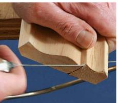
It's not easy to turn corners when sawing at such a steep angle, so the best strategy is to cut as far as you can from one end, back the blade out, and sneak up on the cut from another direction.
