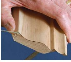
Work inward from both edges to ensure that the last saw stroke separates the meaty center of the molding rather than the fragile outer edge.
