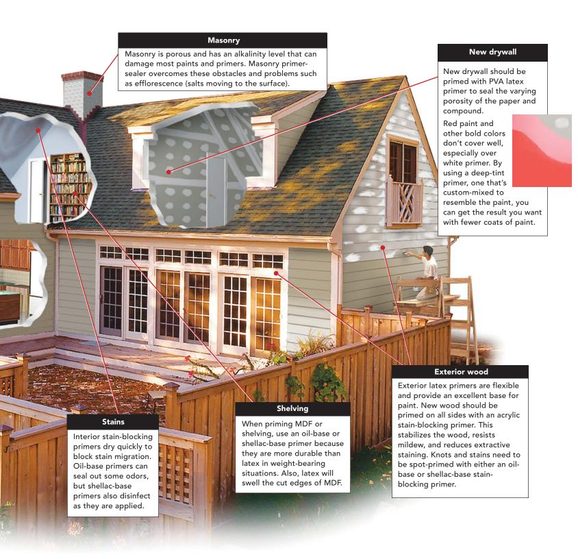
blocking primer. Because oil-base primers are so inflexible (brittle is how one painter describes them), painters are now using 100% acrylic latex stain-blocking primers. Any waterborne stains will show up immediately, and they can be spot-primed with an oil-base stain-blocking primer without inhibiting the flexibility of the latex.
