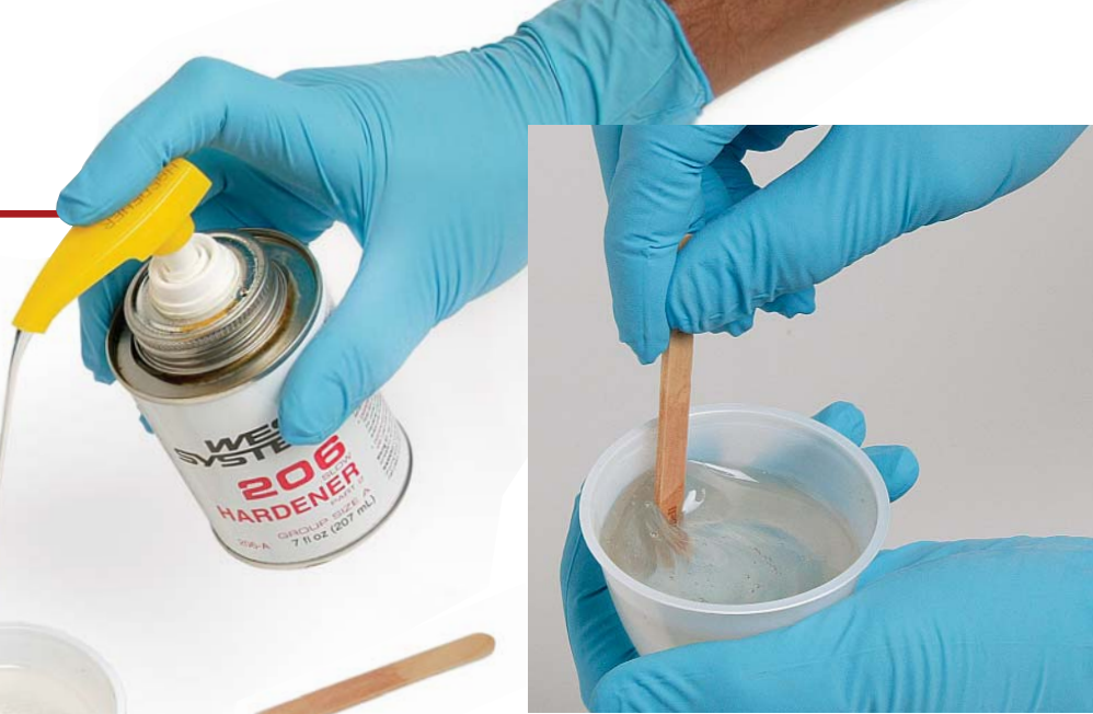
It starts as a liquid. One squirt each of the resin and hardener components is pumped into a clean container, and the epoxy is stirred vigorously for at least one minute.
