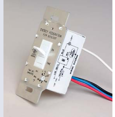
Delay-timer switch keeps the fan running until the steam clears.
