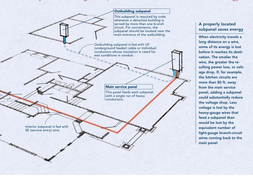
very modern house has a main electrical panel that houses the circuit breakers. These days, many houses also have a secondary breaker panel, commonly called a subpanel. This setup—two power-distribution centers—offers real advantages in some situations. If you understand a few key differences between the wiring in a main panel and that in a subpanel, installing a subpanel can be an easy way to improve the convenience as well as the overall performance of a home's electrical system.
