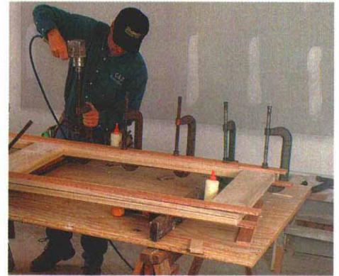
Air-powered impact driver speeds clamping. Hex nuts welded to clamp screws accommodate the driver. A few brads keep the frames from sliding out of place.
